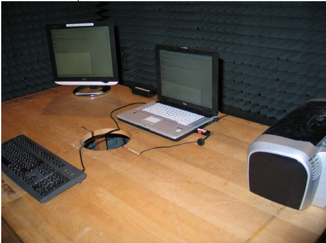
Photo 2: Test setup for radiated measurements
