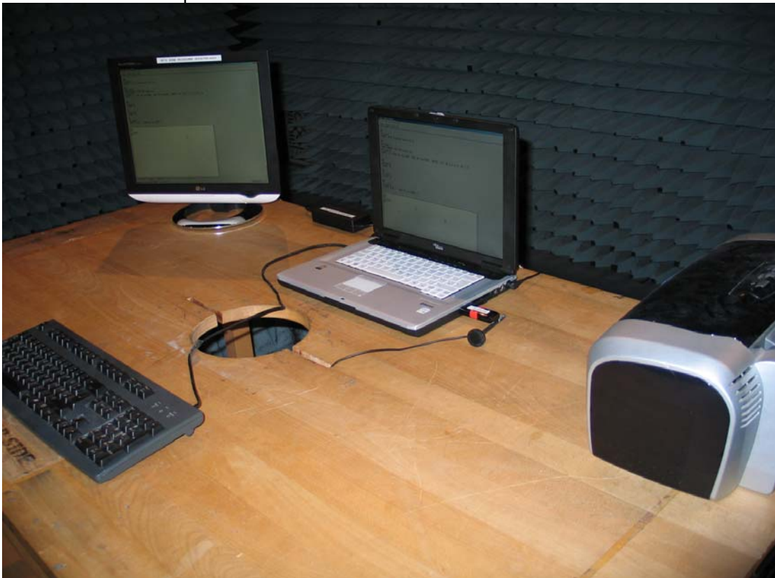
Photo 2: Test setup for radiated measurements
