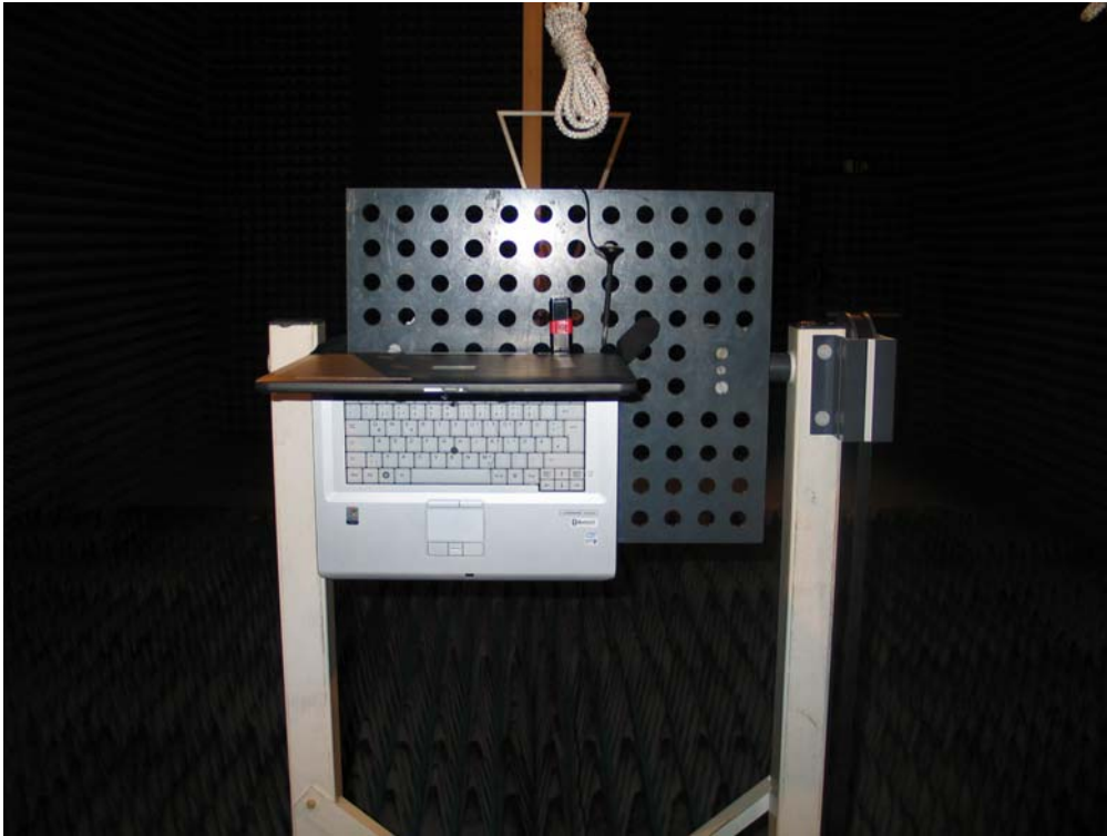
Photo 5: Setup for radiated measurement
