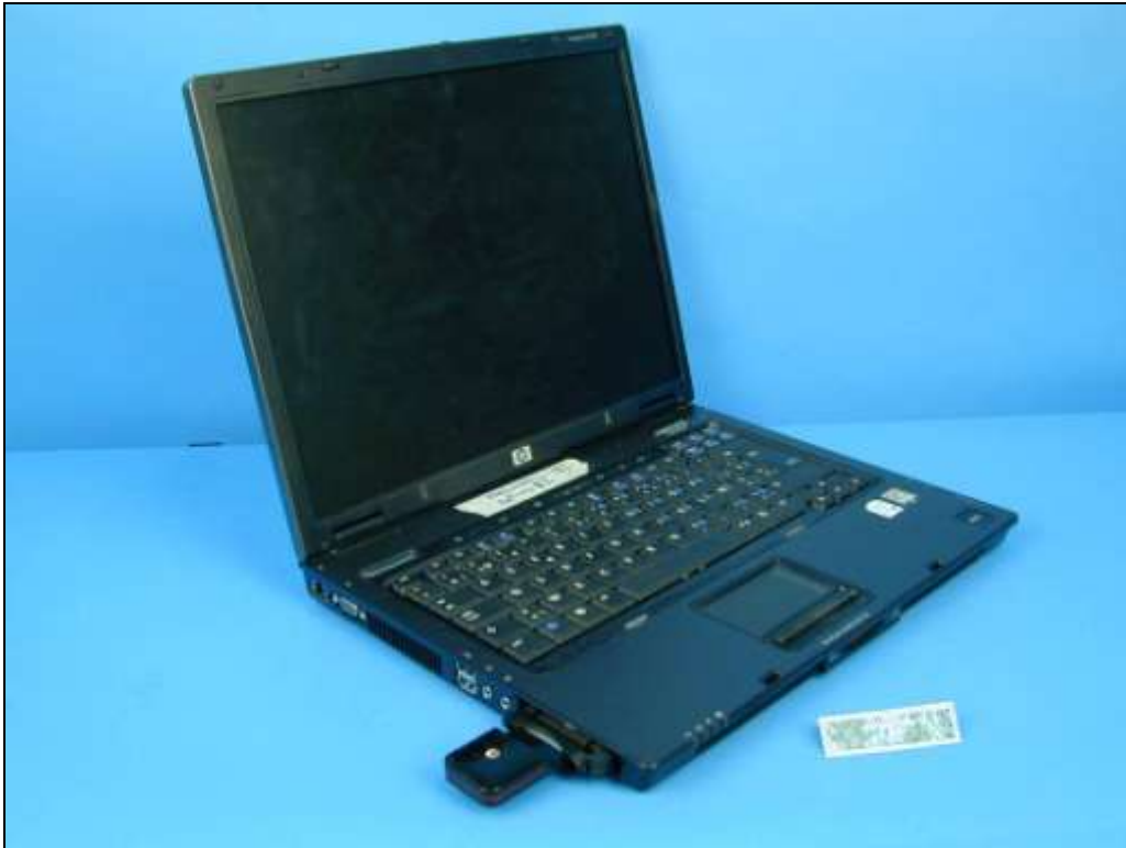
Figure 36: Front View of GE0421 Express Card and adapter connected to Host Laptop: HP Compaq nc 6320
