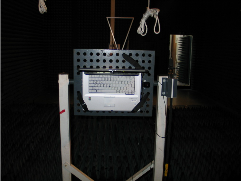
Photo 3: Setup for radiated tests
