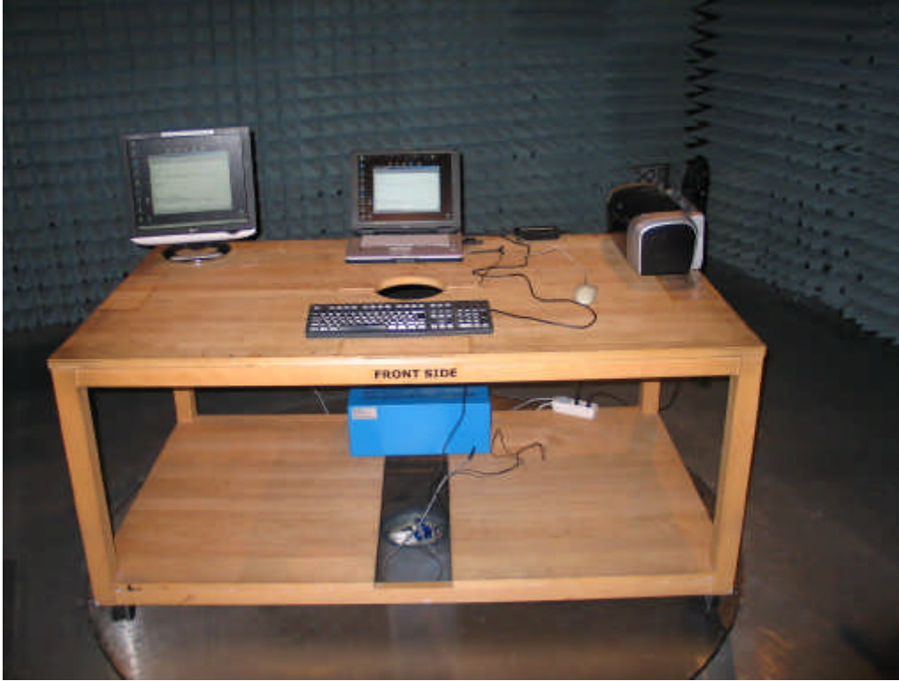
Photo 1: Test setup for radiated measurements
