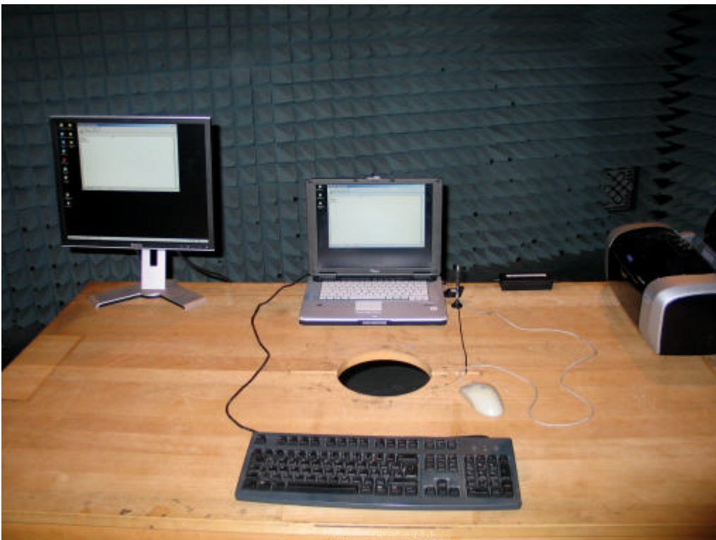
Photo 2: Test setup for radiated measurements
