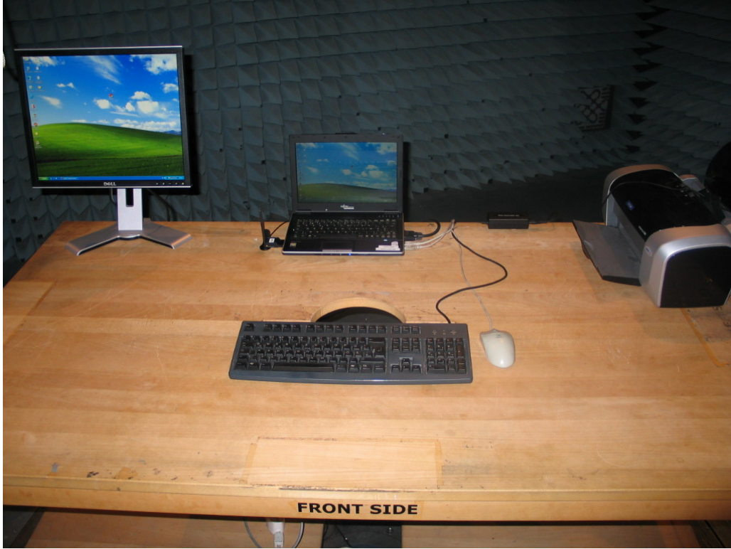
Photo 1: Test setup for radiated measurements
