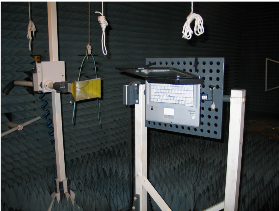
Photo 4: Test setup a01 in the anechoic chamber
