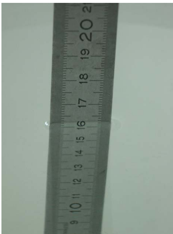
Fig. 28: Liquid depth for GPRS 1900 and WCDMA II Body measurements.
