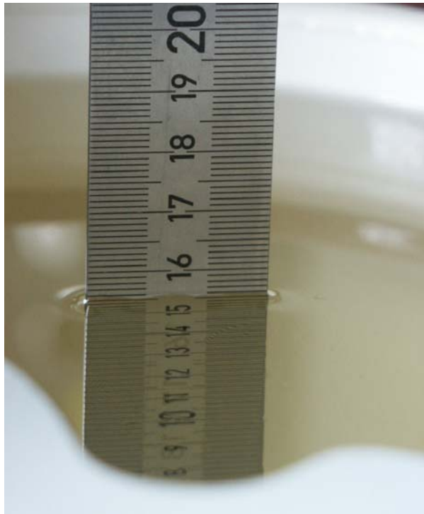
Fig. 27: Liquid depth for GPRS 850 and WCDMA V Body measurements.
