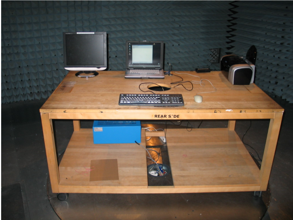
Photo 2: Test setup for radiated measurements
