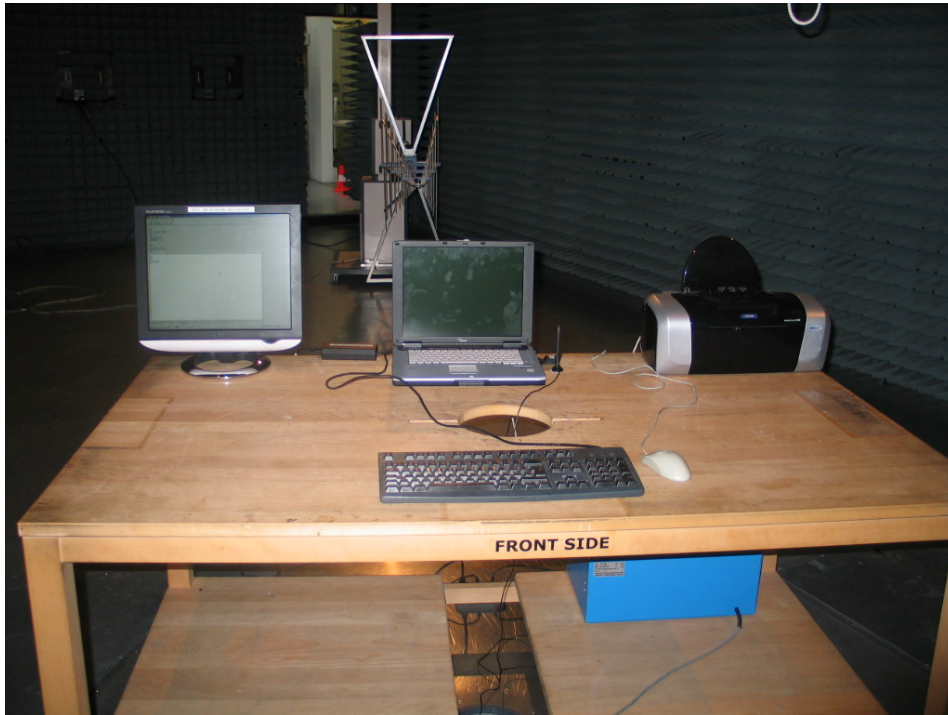
Photo 1: Test setup for radiated measurements
