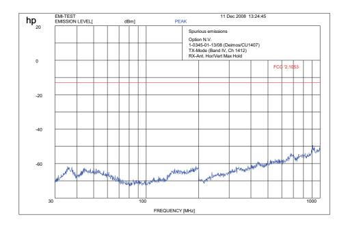
$f \le 1 \text{ GHz}: RBW/VBW: 100 \text{ kHz}$
