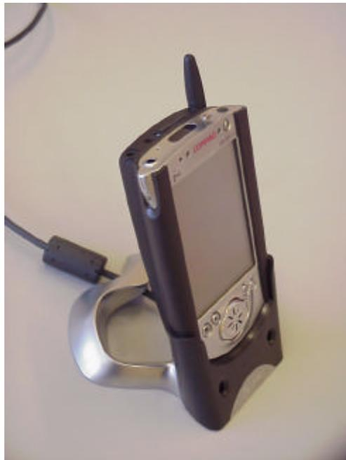
When your Wireless Pack is on, the charge icon appears in the software application while your Wireless Pack charges. Note that your Wireless Pack must be in your handheld while charging, and that it takes about 90 minutes to charge the battery. It's time to recharge the battery when you observe one of the following:
