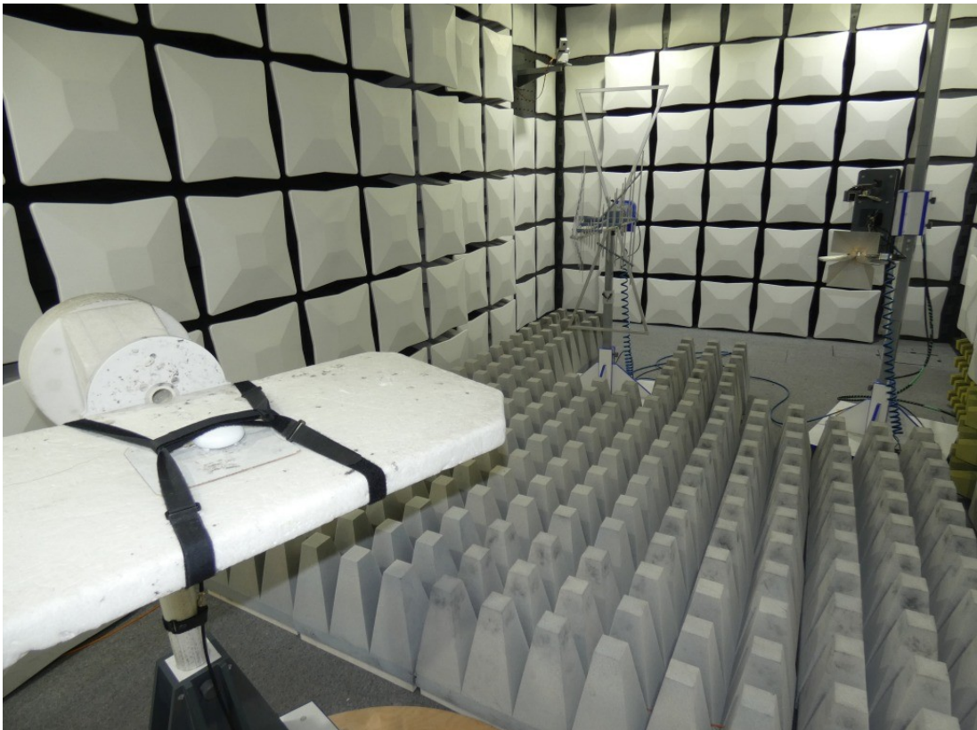
Photo 3: Test setup for radiated measurements above 1 GHz
