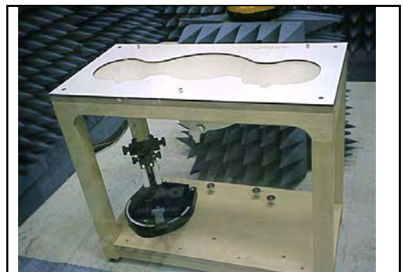
Figure 6. SAM Twin Phantom
