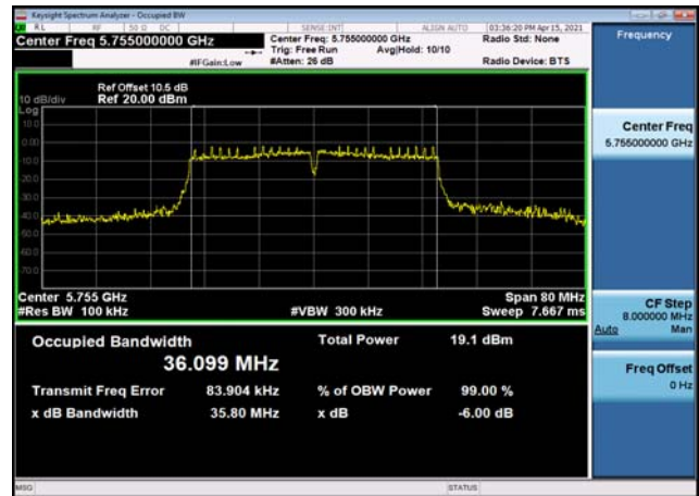
U-NII-3 6dB Bandwidth-802.11ac(80MHz) ,5775MHz,Ant1
