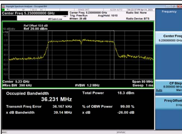
U-NII-1 26dB Bandwidth-802.11n(40MHz) ,5230MHz,Ant1
