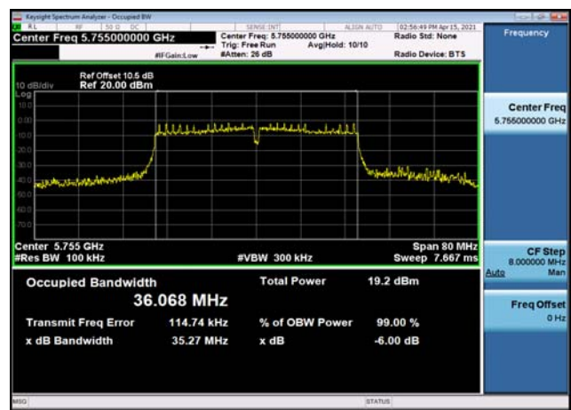
U-NII-3 6dB Bandwidth-802.11n(40MHz),5755MHz,Ant1
