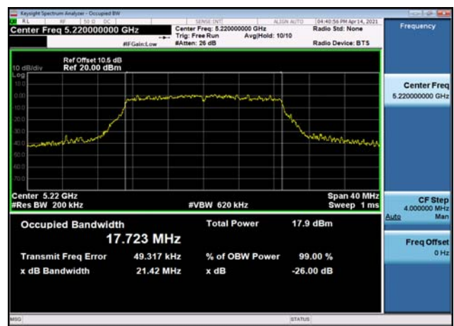
U-NII-1 26dB Bandwidth-802.11n(40MHz) ,5190MHz,Ant1
