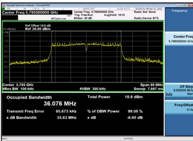
U-NII-3 6dB Bandwidth-802.11a(20MHz) ,5785MHz,Ant1
