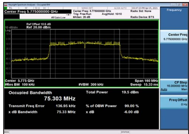
U-NII-3 6dB Bandwidth-802.11ac(80MHz) ,5775MHz,Ant1
