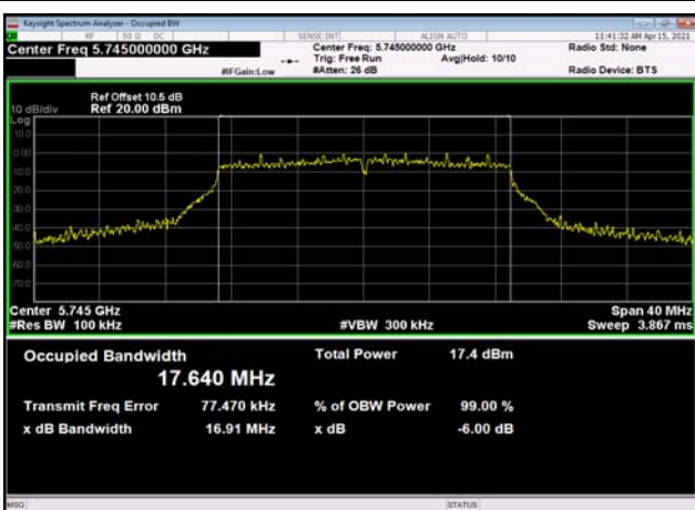
U-NII-3 6dB Bandwidth-802.11ac(20MHz) ,5745MHz,Ant1
