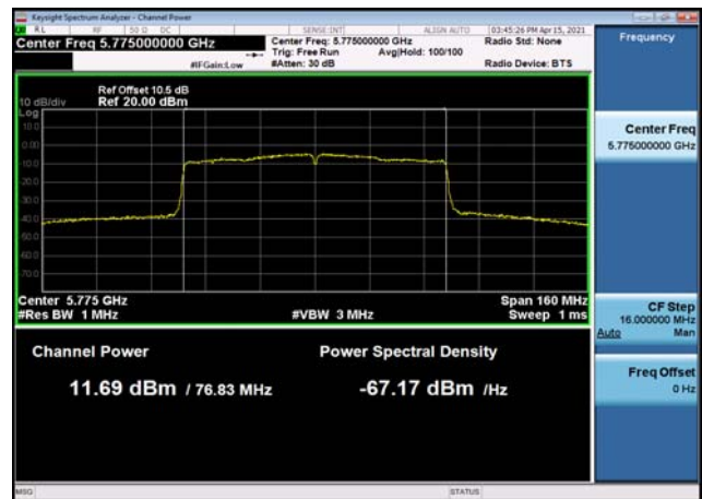
U-NII-3 Output Power-802.11ac(80MHz) ,5775MHz,Ant1
