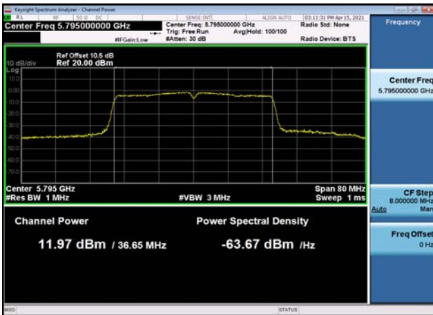
U-NII-3 Output Power-802.11a(20MHz) ,5785MHz,Ant1
