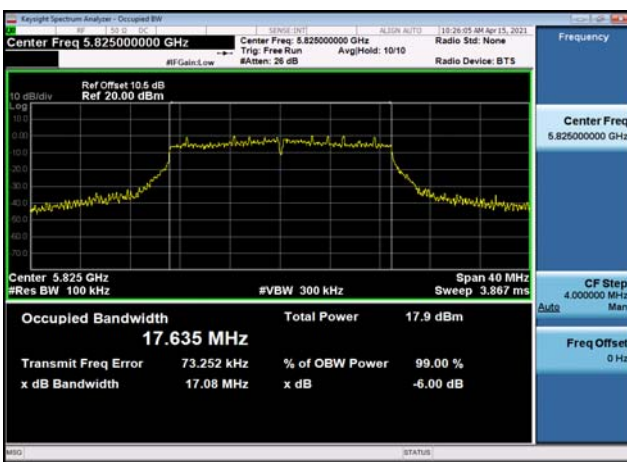
U-NII-3 6dB Bandwidth-802.11n(20MHz),5825MHz,Ant1
