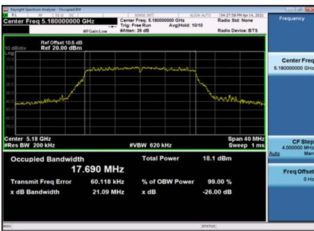
U-NII-1 26dB Bandwidth-802.11n(20MHz) ,5240MHz,Ant1
