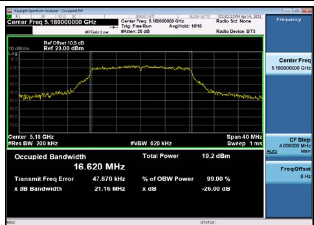
U-NII-1 26dB Bandwidth-802.11a(20MHz) ,5180MHz,Ant1
