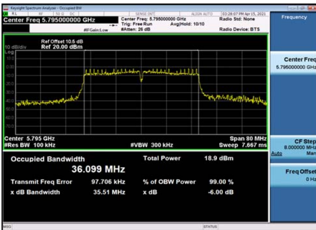
U-NII-3 6dB Bandwidth-802.11ac(40MHz) ,5795MHz,Ant1
