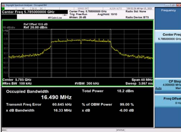
U-NII-3 6dB Bandwidth-802.11ac(20MHz) ,5745MHz,Ant1
