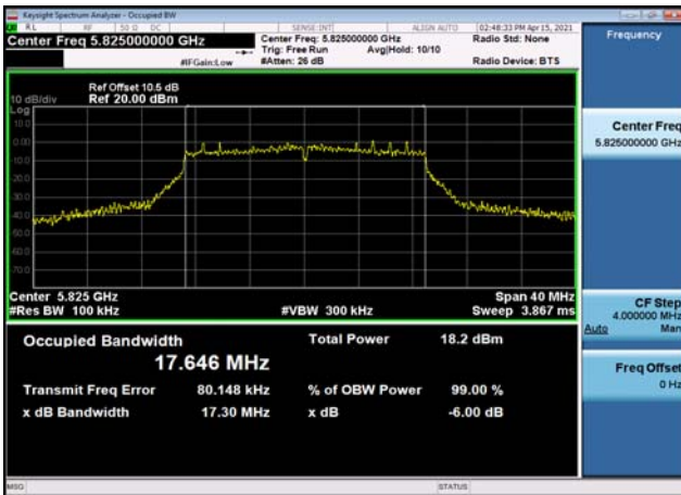
U-NII-3 6dB Bandwidth-802.11ac(40MHz) ,5795MHz,Ant1
