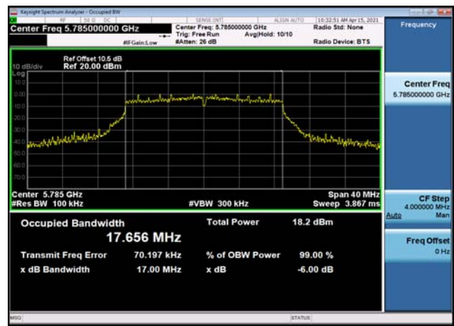
U-NII-3 6dB Bandwidth-802.11n(40MHz),5755MHz,Ant1
