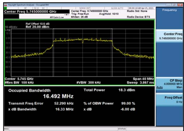
U-NII-3 6dB Bandwidth-802.11a(20MHz) ,5825MHz,Ant1
