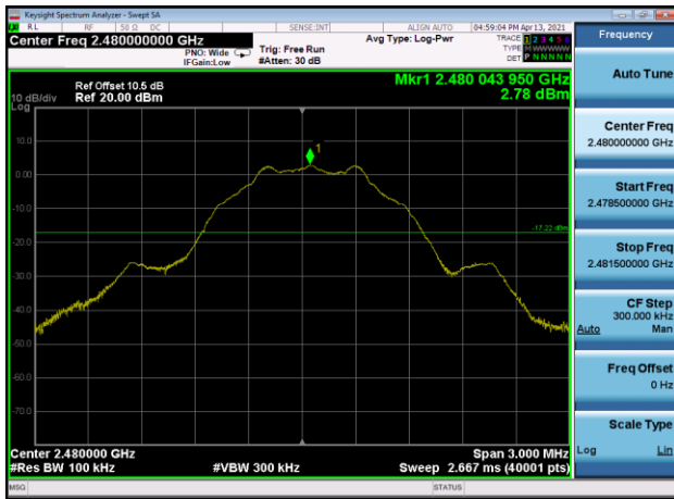
,Plot ,2Conducted Emission: 2440 ,Band Edge
