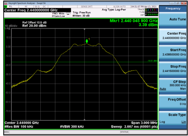
,Plot ,2Conducted Emission: 2402 ,Band Edge
