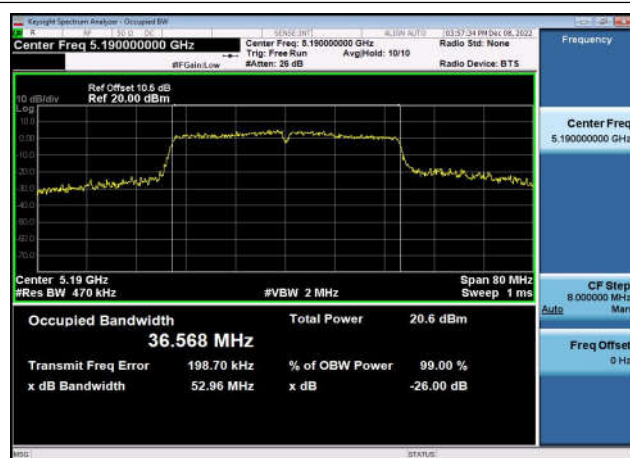
U-NII-1 26dB & 99% Bandwidth-802.11ac(40MHz) ,5190MHz,Ant1
