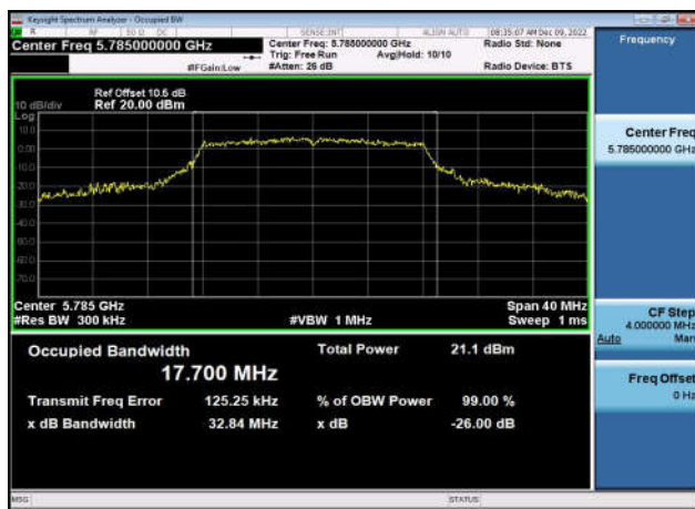
U-NII-3 26dB & 99% Bandwidth-802.11ac(20MHz) ,5745MHz,Ant1
