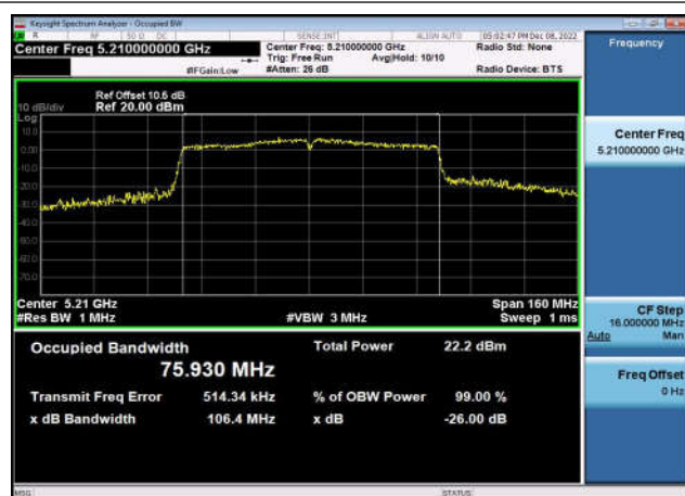
U-NII-3 26dB & 99% Bandwidth-802.11n(20MHz),5785MHz,Ant1
