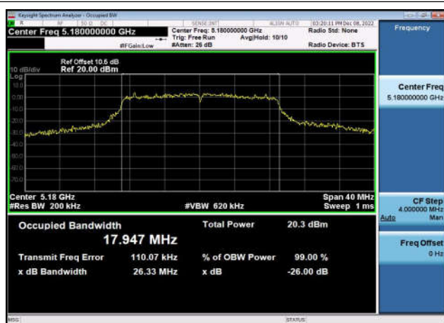
U-NII-1 26dB & 99% Bandwidth-802.11ac(20MHz) ,5240MHz,Ant1
