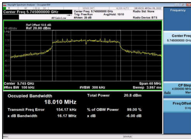
U-NII-3 6dB Bandwidth-802.11n(20MHz) ,5825MHz,Ant1
