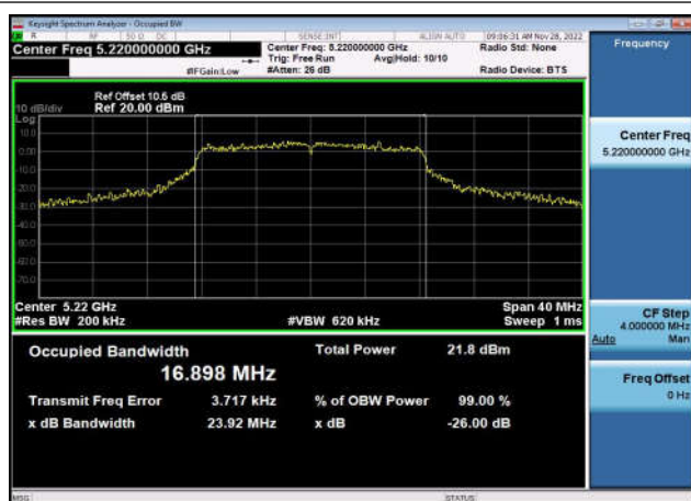
U-NII-1 26dB & 99% Bandwidth-802.11ac(20MHz) ,5180MHz,Ant1
