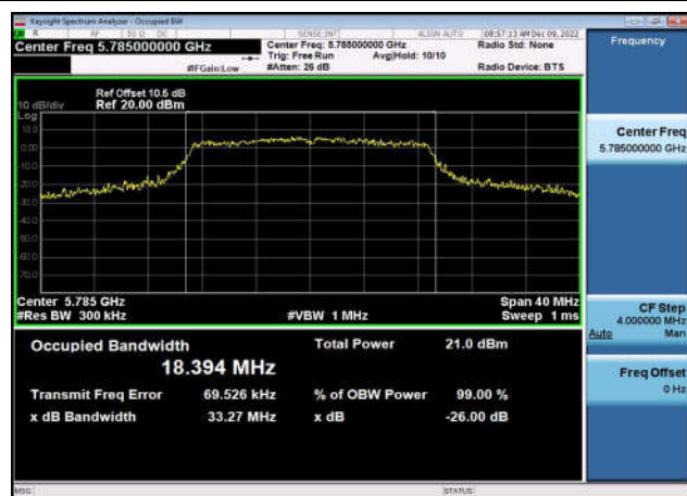
U-NII-3 26dB & 99% Bandwidth-802.11n(40MHz),5755MHz,Ant1
