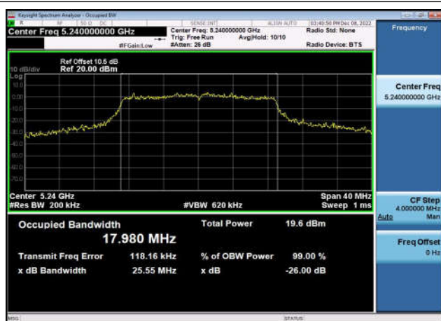
U-NII-1 26dB & 99% Bandwidth-802.11ac(20MHz) ,5240MHz,Ant1
