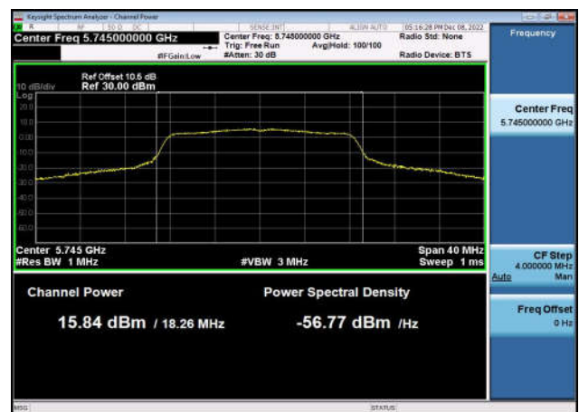
U-NII-3 Output Power-802.11a(20MHz) ,5825MHz,Ant1
