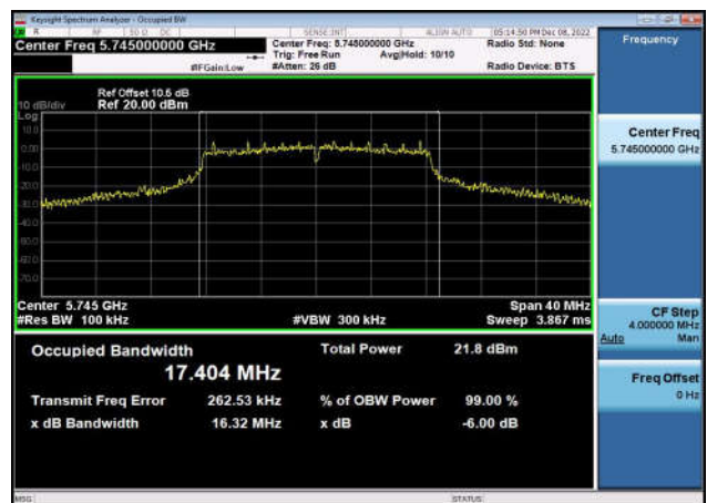
U-NII-3 6dB Bandwidth-802.11a(20MHz) ,5745MHz,Ant1
