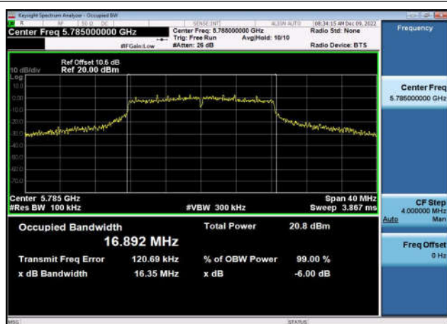
U-NII-3 6dB Bandwidth-802.11ac(20MHz) ,5745MHz,Ant1
