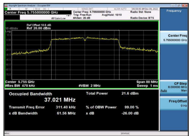
U-NII-3 26dB & 99% Bandwidth-802.11ac(80MHz) ,5775MHz,Ant1
