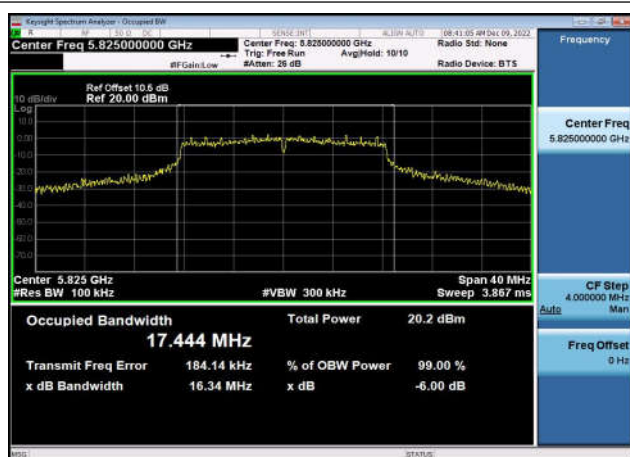
U-NII-3 6dB Bandwidth-802.11ac(20MHz) ,5785MHz,Ant1
