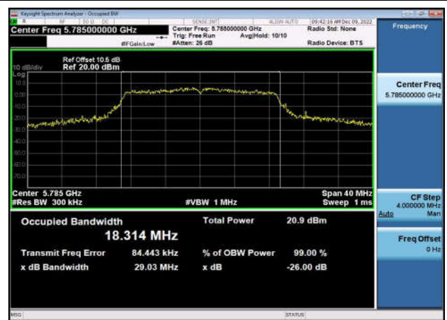
U-NII-3 26dB & 99% Bandwidth-802.11ac(20MHz) ,5785MHz,Ant1
