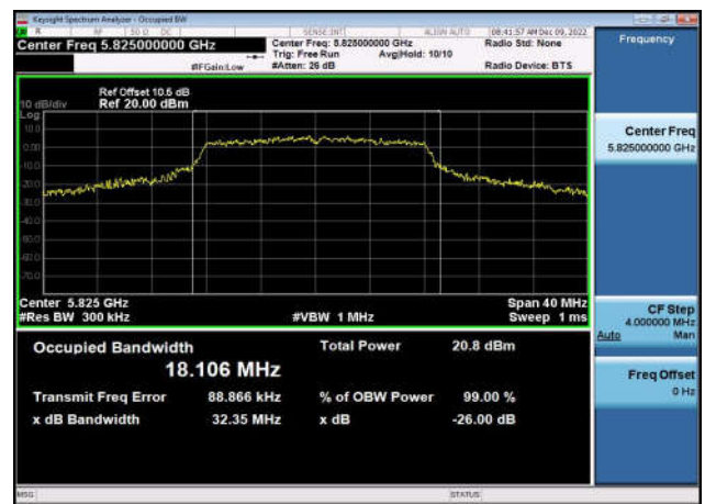
U-NII-3 26dB & 99% Bandwidth-802.11ac(20MHz) ,5785MHz,Ant1
