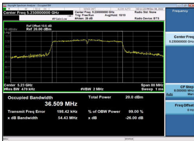
U-NII-1 26dB & 99% Bandwidth-802.11n(40MHz) ,5230MHz,Ant1
