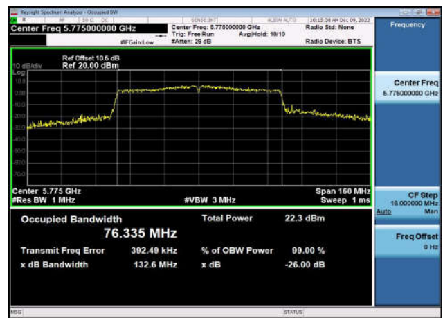
U-NII-3 26dB & 99% Bandwidth-802.11ac(80MHz) ,5775MHz,Ant1
