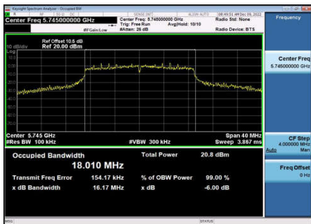
U-NII-3 6dB Bandwidth-802.11n(20MHz) ,5825MHz,Ant1
