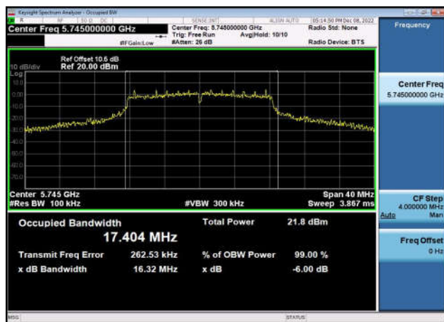
U-NII-3 6dB Bandwidth-802.11a(20MHz) ,5745MHz,Ant1
