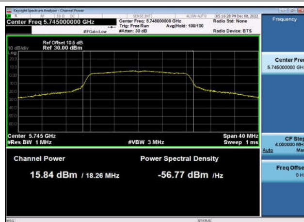
U-NII-3 Output Power-802.11a(20MHz) ,5825MHz,Ant1
