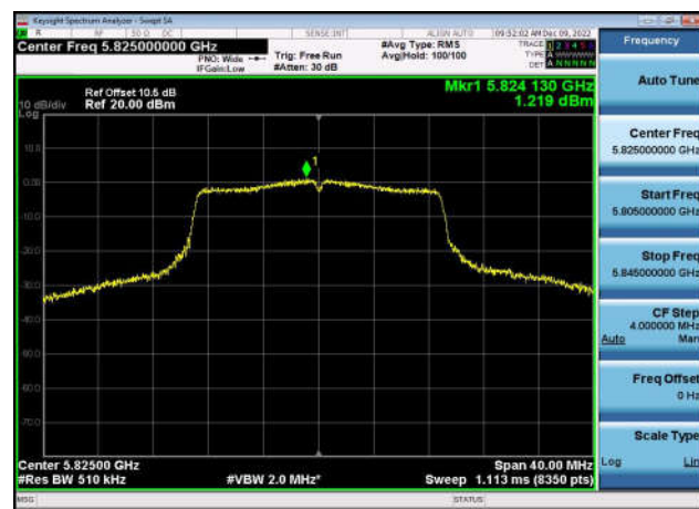
U-NII-3 Power spectral density-802.11 ac(40MHz),5795MHz,Ant1
