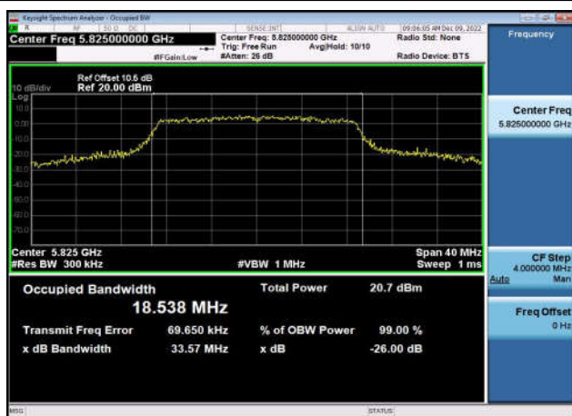
U-NII-3 26dB & 99% Bandwidth-802.11n(20MHz),5825MHz,Ant1
