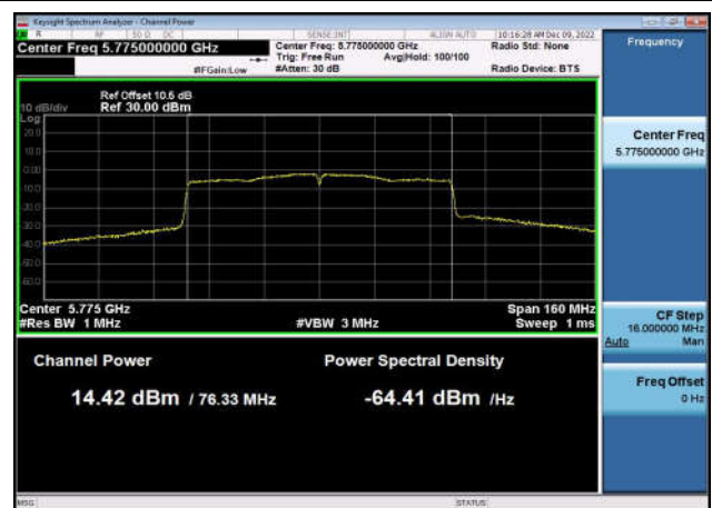
U-NII-3 Output Power-802.11ac(80MHz) ,5775MHz,Ant1
