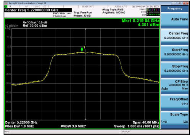
U-NII-1 Power spectral density-802.11 n(40MHz),5190MHz,Ant1
