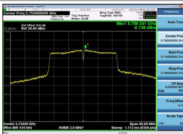
U-NII-3 Power spectral density-802.11 n(40MHz),5755MHz,Ant1
