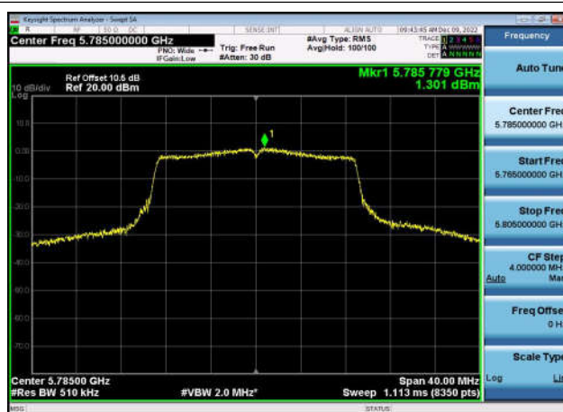
U-NII-3 Power spectral density-802.11 ac(20MHz),5785MHz,Ant1
