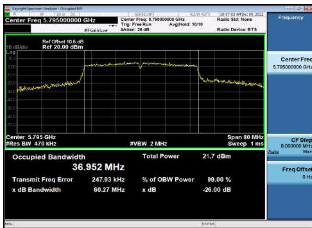
U-NII-3 26dB & 99% Bandwidth-802.11ac(40MHz) ,5795MHz,Ant1
