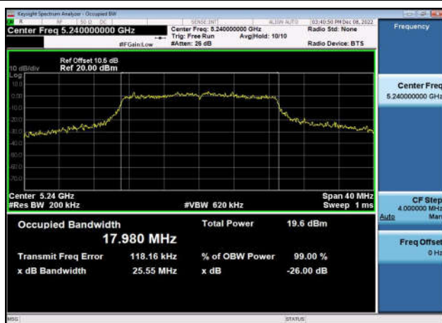
U-NII-1 26dB & 99% Bandwidth-802.11ac(20MHz) ,5240MHz,Ant1
