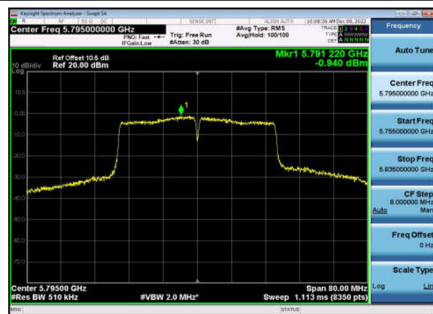
U-NII-3 Power spectral density-802.11 ac(40MHz),5795MHz,Ant1
