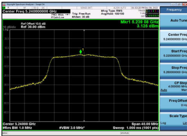
U-NII-1 Power spectral density-802.11 n(40MHz),5230MHz,Ant1
