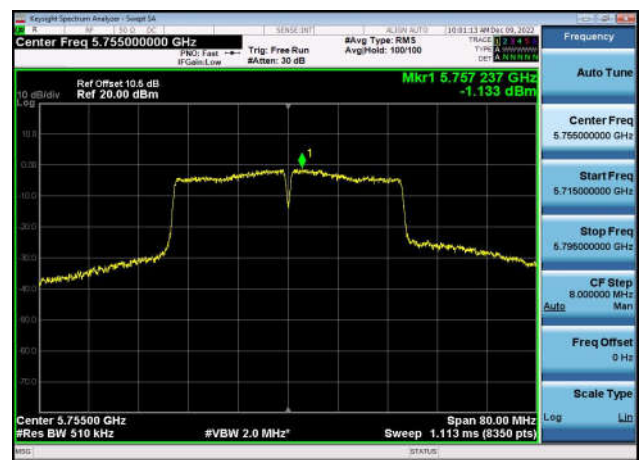
U-NII-3 Power spectral density-802.11 ac(80MHz),5775MHz,Ant1
