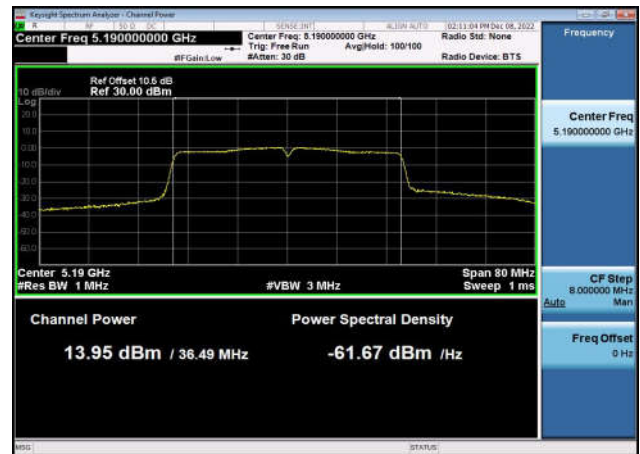
U-NII-1 Output Power-802.11a(20MHz) ,5180MHz,Ant1
