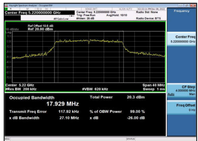
U-NII-1 26dB & 99% Bandwidth-802.11ac(40MHz) ,5190MHz,Ant1
