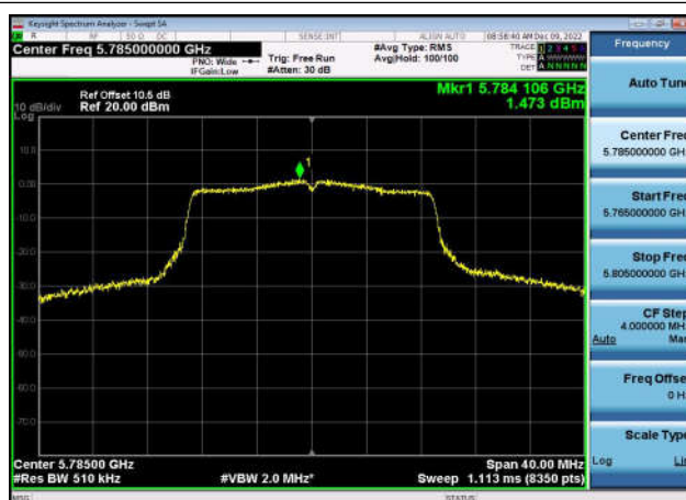
U-NII-3 Power spectral density-802.11 n(40MHz),5755MHz,Ant1
