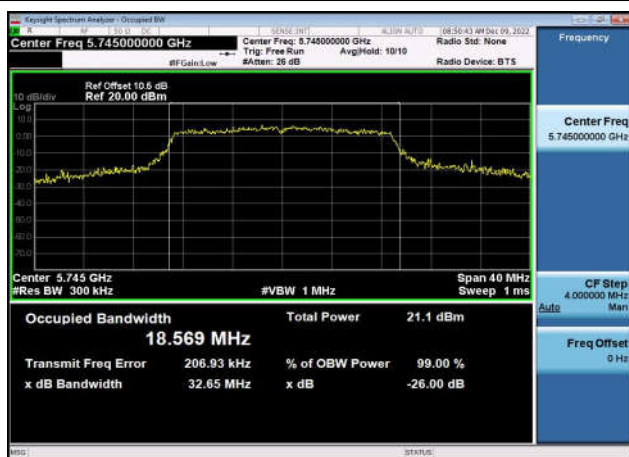
U-NII-3 26dB & 99% Bandwidth-802.11n(20MHz),5825MHz,Ant1
