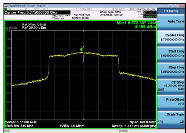
U-NII-3 Power spectral density-802.11 ac(80MHz),5775MHz,Ant1
