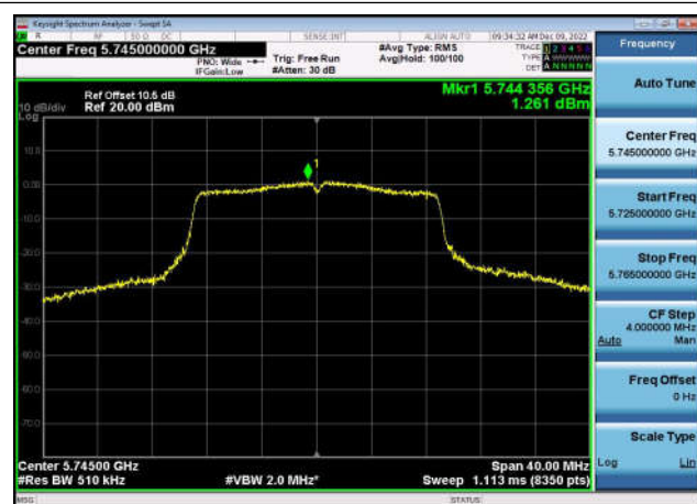
U-NII-3 Power spectral density-802.11 ac(20MHz),5745MHz,Ant1
