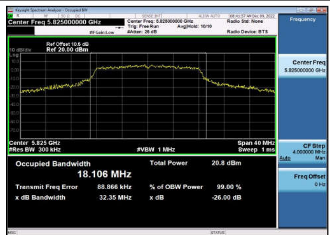
U-NII-3 26dB & 99% Bandwidth-802.11ac(20MHz) ,5785MHz,Ant1
