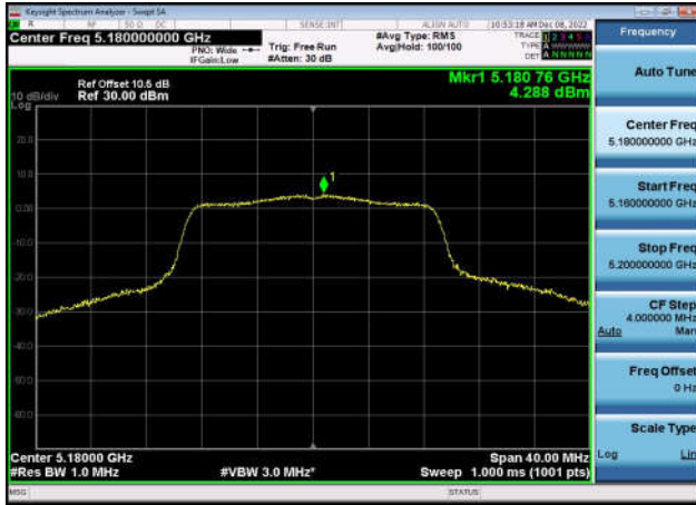
U-NII-1 Power spectral density-802.11 n(20MHz),5240MHz,Ant1
