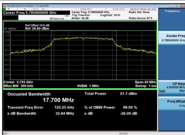
U-NII-3 26dB & 99% Bandwidth-802.11ac(20MHz) ,5745MHz,Ant1
