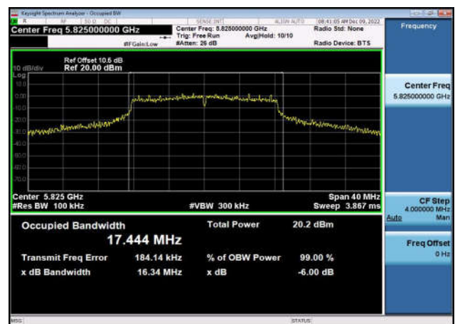
U-NII-3 6dB Bandwidth-802.11ac(20MHz) ,5785MHz,Ant1
