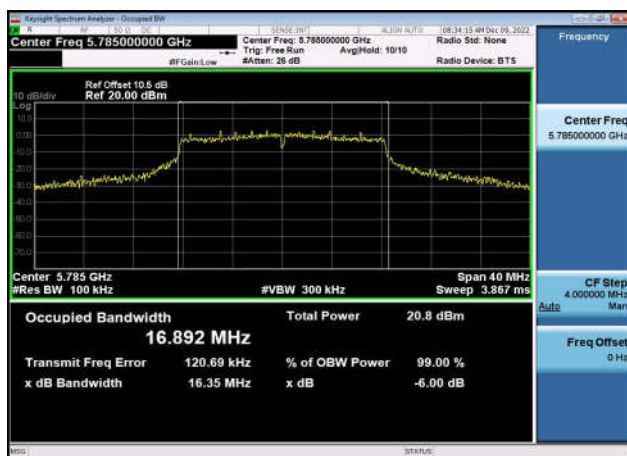
U-NII-3 6dB Bandwidth-802.11ac(20MHz) ,5745MHz,Ant1
