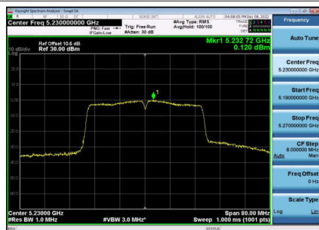
U-NII-3 Power spectral density-802.11 n(20MHz),5745MHz,Ant1
