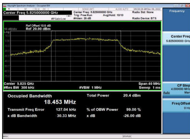
U-NII-3 26dB & 99% Bandwidth-802.11ac(40MHz) ,5795MHz,Ant1
