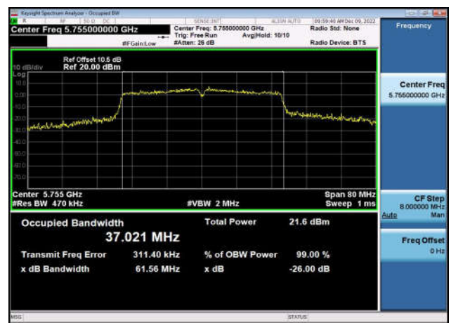
U-NII-3 26dB & 99% Bandwidth-802.11ac(80MHz) ,5775MHz,Ant1
