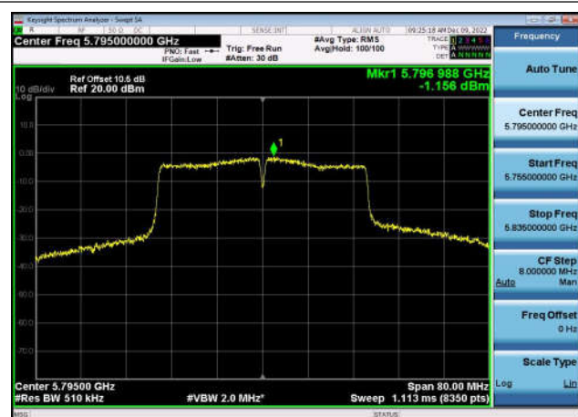
U-NII-3 Power spectral density-802.11 a(20MHz),5785MHz,Ant1
