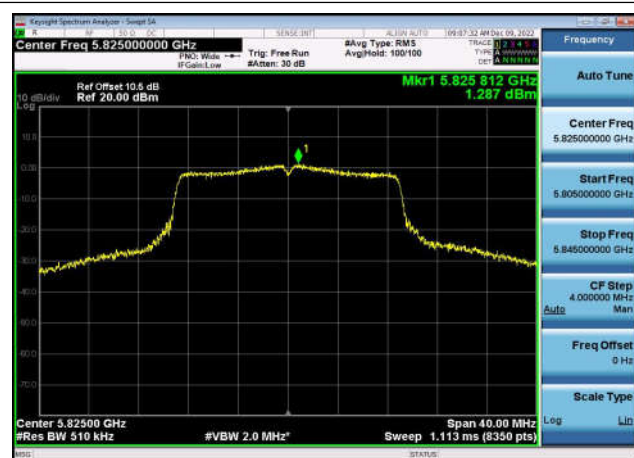
U-NII-3 Power spectral density-802.11 n(20MHz),5825MHz,Ant1
