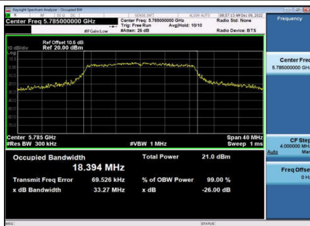
U-NII-3 26dB & 99% Bandwidth-802.11n(40MHz),5755MHz,Ant1
