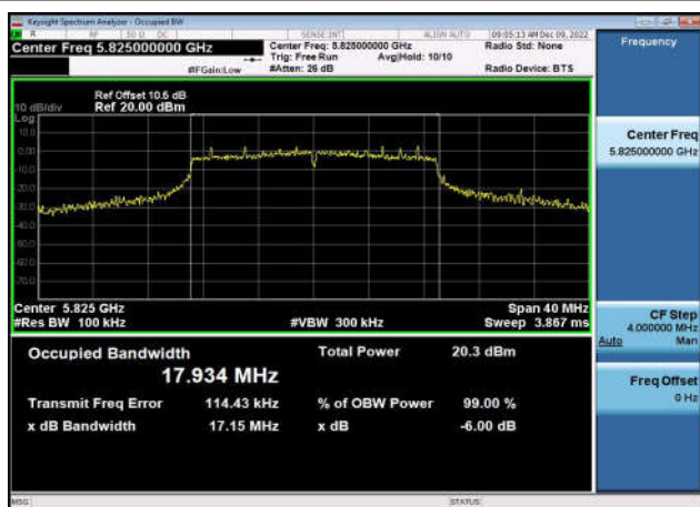
U-NII-3 6dB Bandwidth-802.11n(40MHz) ,5795MHz,Ant1
