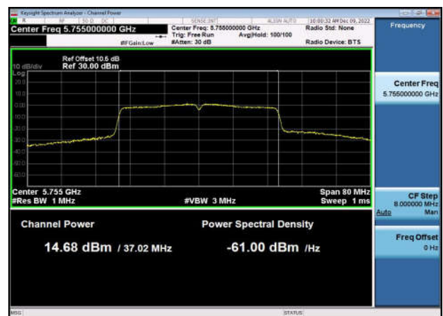
U-NII-3 Output Power-802.11ac(80MHz) ,5775MHz,Ant1
