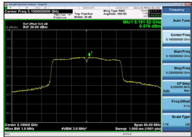
U-NII-1 Power spectral density-802.11 a(20MHz),5180MHz,Ant1
