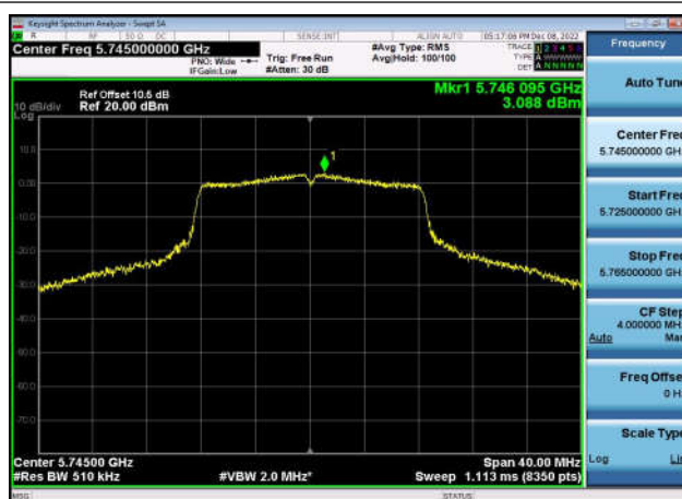
U-NII-3 Power spectral density-802.11 a(20MHz),5825MHz,Ant1
