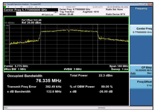
U-NII-3 26dB & 99% Bandwidth-802.11ac(80MHz) ,5775MHz,Ant1
