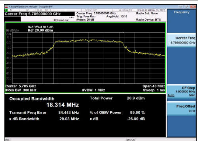
U-NII-3 26dB & 99% Bandwidth-802.11ac(20MHz) ,5785MHz,Ant1
