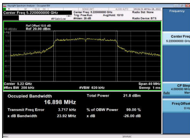
U-NII-1 26dB & 99% Bandwidth-802.11ac(20MHz) ,5180MHz,Ant1
