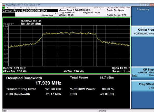
U-NII-1 26dB & 99% Bandwidth-802.11n(40MHz) ,5230MHz,Ant1
