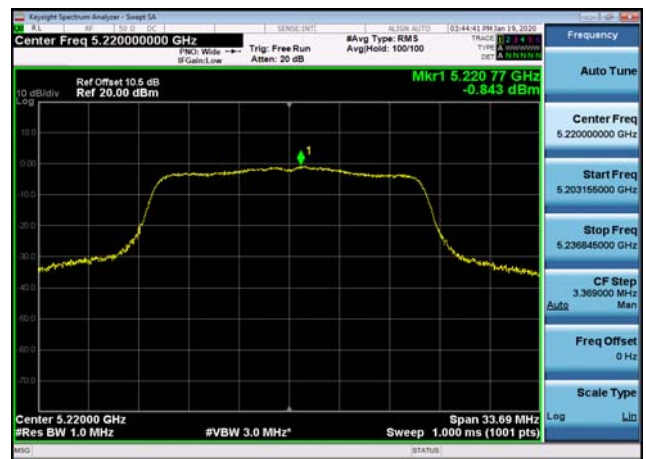
U-NII-1 Power spectral density-802.11 ac(40MHz),5190MHz,Ant1
