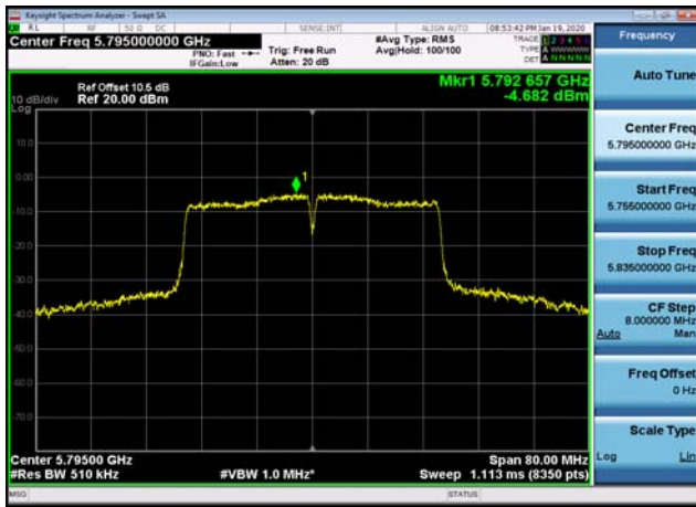
U-NII-3 Power spectral density-802.11 ac(40MHz),5795MHz
