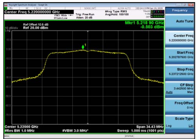
U-NII-1 Power spectral density-802.11 n(40MHz),5190MHz,Ant1
