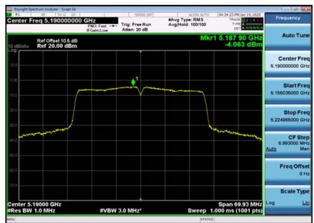
U-NII-1 Power spectral density-802.11 ac(40MHz),5190MHz,Ant1
