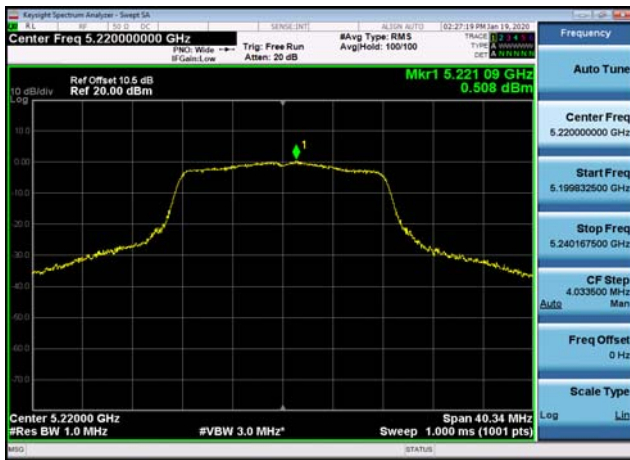
U-NII-1 Power spectral density-802.11 ac(20MHz),5180MHz,Ant1
