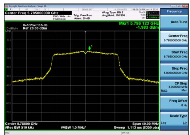
U-NII-3 Power spectral density-802.11 ac(20MHz),5785MHz,Ant1
