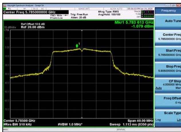
U-NII-3 Power spectral density-802.11 ac(20MHz),5745MHz,Ant1
