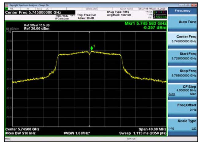
U-NII-3 Power spectral density-802.11 a(20MHz),5825MHz
