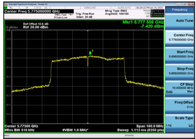
U-NII-3 Power spectral density-802.11 ac(80MHz),5775MHz
