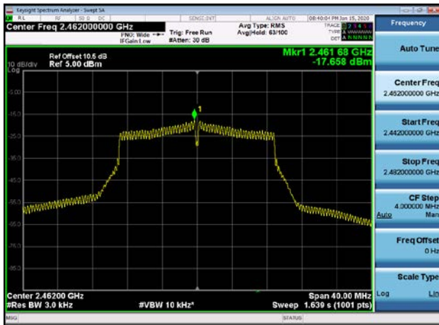
Power spectral density-802.11n(HT20) ,2462MHz,Ant0
