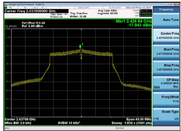
Power spectral density-802.11n(HT20) ,2437MHz,Ant0
