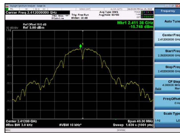
Power spectral density-802.11b ,2462MHz,Ant0
