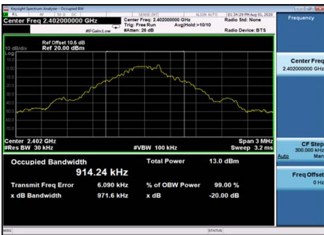
20dB Bandwidth: GFSK,2480MHz,DH5
