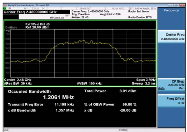
20dB Bandwidth: DQPSK,2480MHz,2DH5
