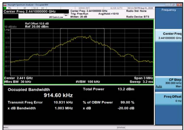
20dB Bandwidth: DQPSK,2402MHz,2DH5
