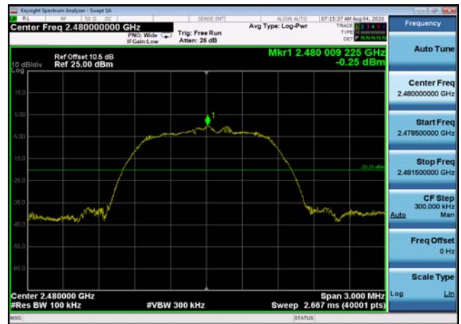
Conducted Emission: DQPSK,2480,2DH5 ,Reference Level
