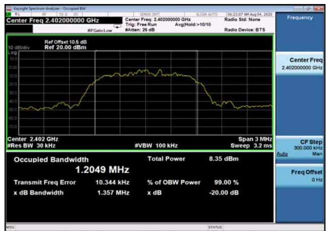
20dB Bandwidth: DQPSK,2480MHz,2DH5
