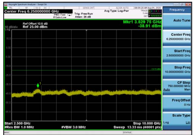
Conducted Emission: 8DPSK,2402,3DH5 ,Band Edge HoppingOFF
