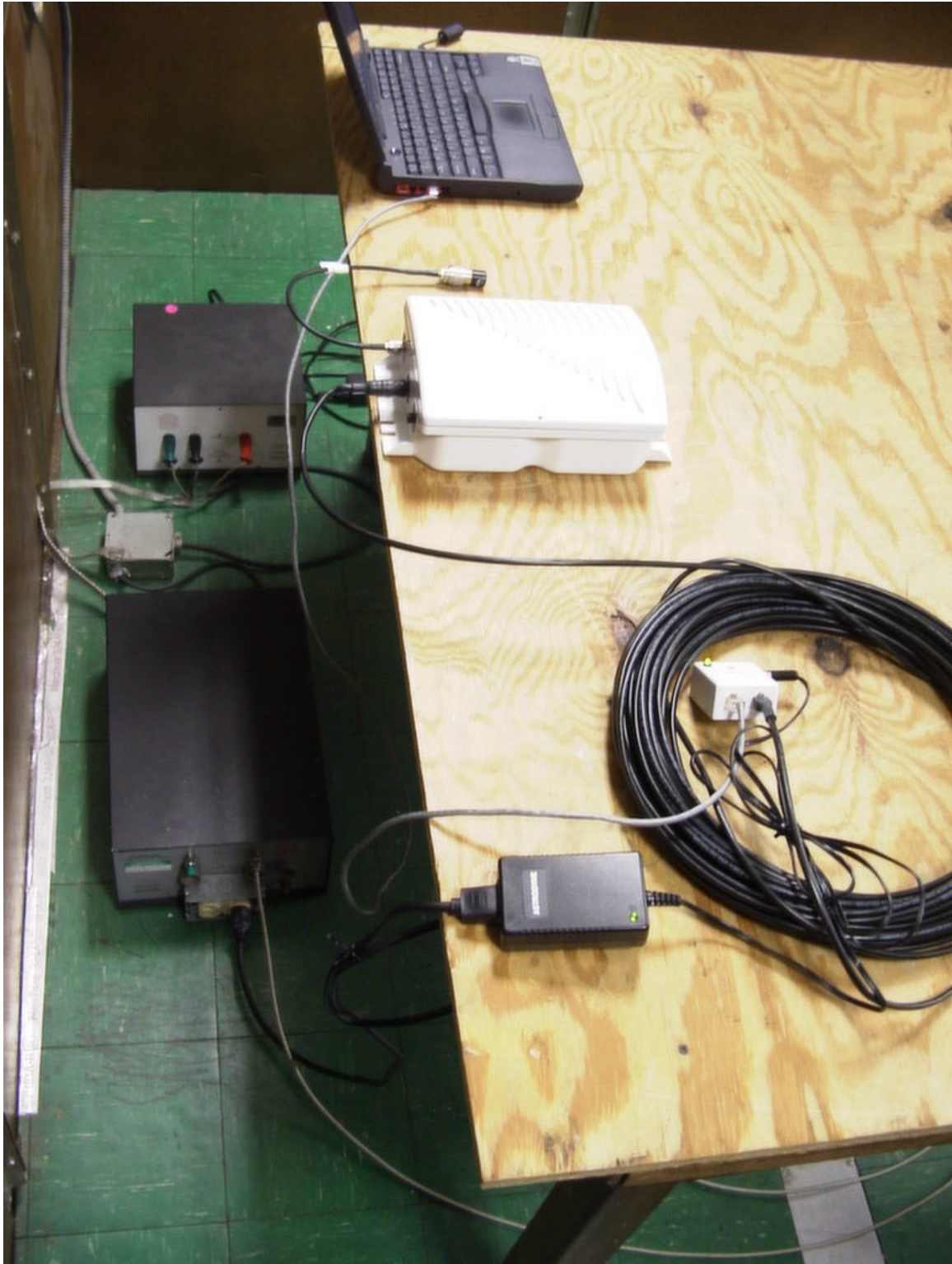
POWERLINE CONDUCTED EMISSIONS TEST SET UP
