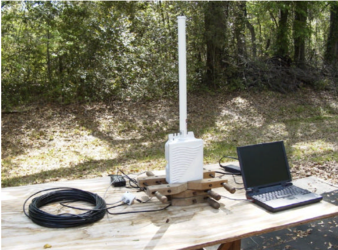
RADIATED EMISSIONS TEST SET UP
