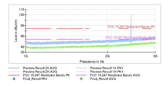
The peak above the limit is the Bluetooth LE carrier frequency.
