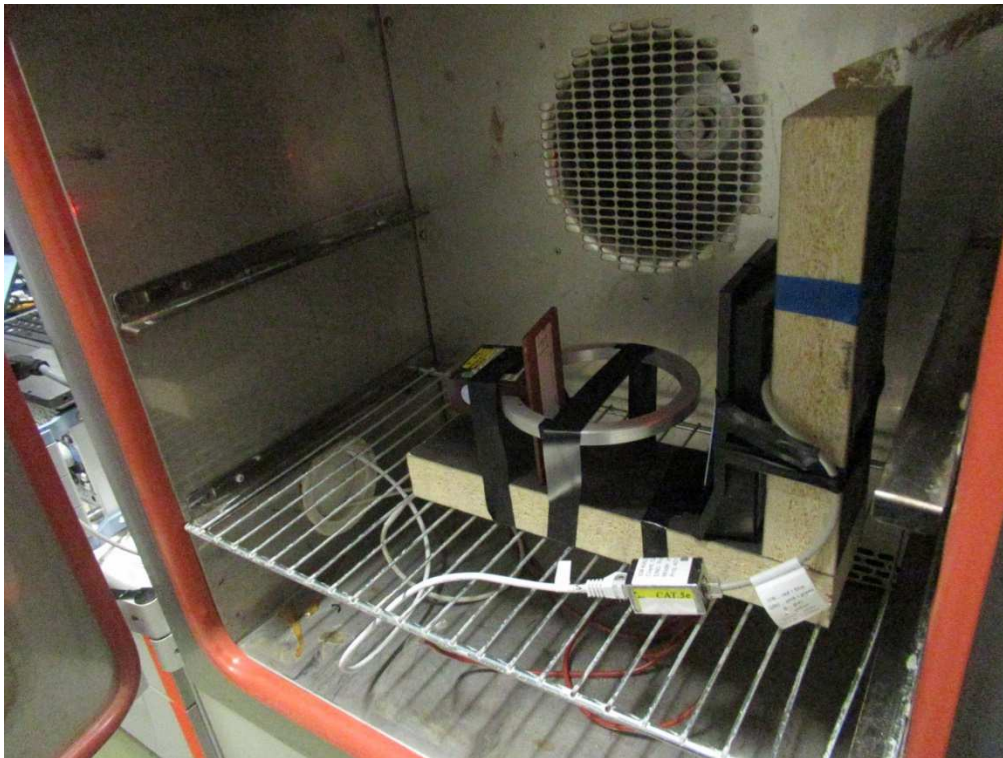
Test Setup Photo – Frequency stability , 20 dB Bandwidth and Occupied Bandwidth
