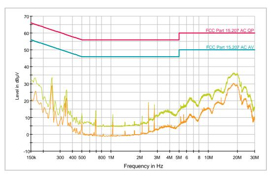
FCC Part 15.207 AC QP [..\EMI conducted\FCC Part 15 Subpart C\]
