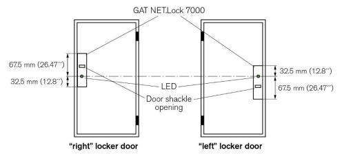
Figure 3.2 - LED positions of the GAT NET.Lock 7020 for right and left-hinged doors
