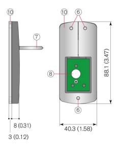
Figure 3.8 - Dimensions of the GAT NET.Lock BoltSet 7320
