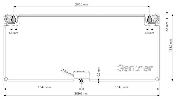
Figure 3.14 - Mounting of the GAT NET. Controller M/S 7020
