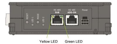
Figure 5.5 - LEDs and buttons on the GAT NET.Controller M 7020
