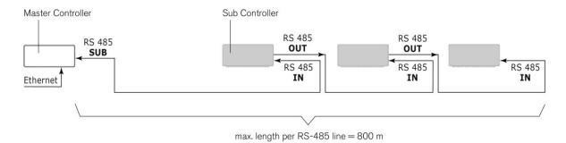
Figure 4.6 – Series connection of the GAT NET.Controller S 7020
