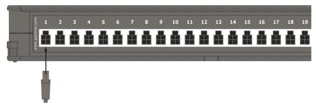
Figure 4.4 - Connecting the GAT NET.Lock 7020 to a GAT NET.Controller S 7020 sub controller
