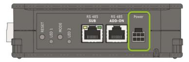
Figure 4.13 - Power supply connection on the GAT NET.Controller M 7020
