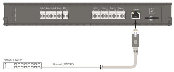
Figure 4.12 - GAT NET. Controller M 7020 Ethernet connection
