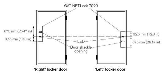
Figure 3.1 - Definition of the opening direction of lockers (left/right)
