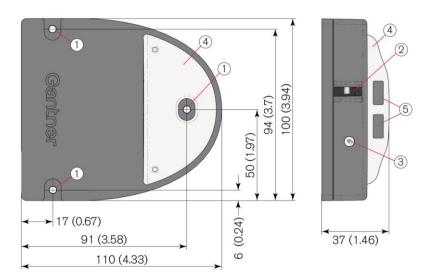
Figure 3.5 - Dimensions of the GAT NET.Lock 7020 USB / GAT NET.Lock 7020 USB P
