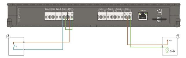
Figure 4.16 - Relay and optocoupler connection example
