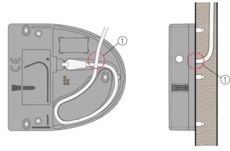
Figure 4.3 - GAT NET.Lock 7020 cable routing
