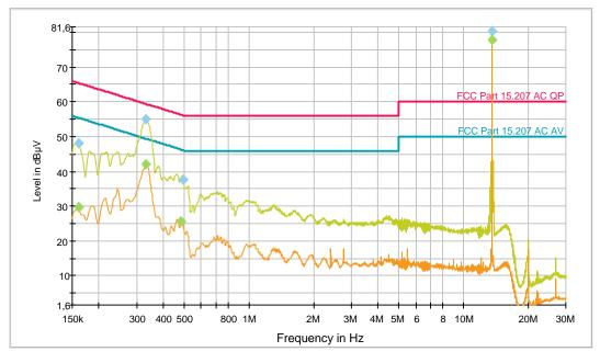
FCC Part 15.207 AC QP [..\EMI conducted\FCC Part 15 Subpart C\] FCC Part 15.207 AC AV [..\EMI conducted\FCC Part 15 Subpart C\] Preview Result 1-QPK [Preview Result 1.Result:1] Preview Result 2-CAV [Preview Result 2.Result:2] Final Result 1-QPK [Final Result 1.Result:1] Final Result 2-CAV [Final Result 2.Result:1]
