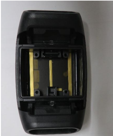
Figure 1 Photograph of the antenna installed in the product
