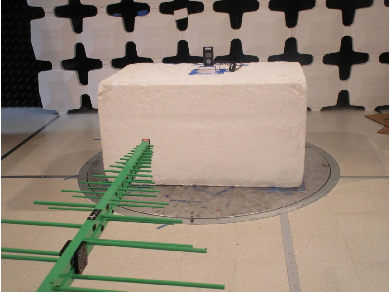
Figure 15: Radiated Emissions – Front View – 30 MHz - 1 GHz – EUT Upright
