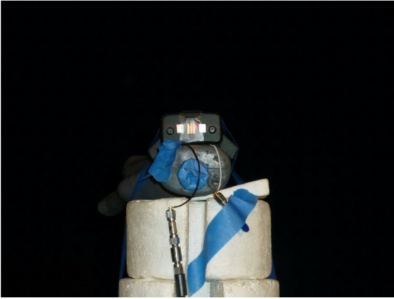
Figure 35 – Test setup in Satimo’s SG64 antenna range
