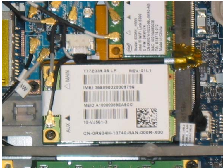
RF Modules Installed
