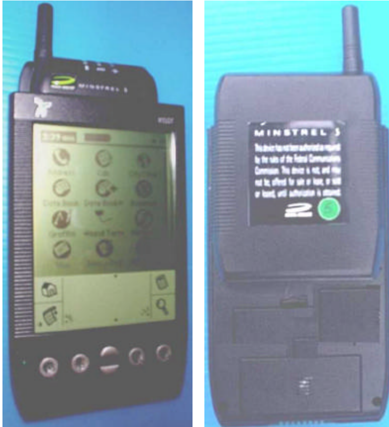
Novatel Wireless Minstrel S wireless CDPD modem installed on Handspring Visor
