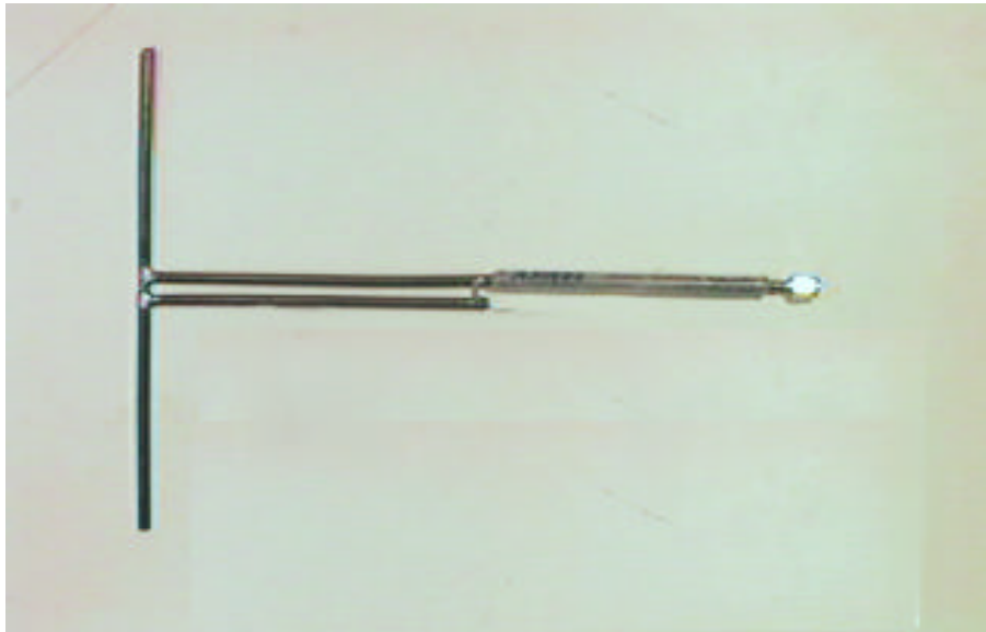
Reference Dipole Antenna Used for ERP Measurement
