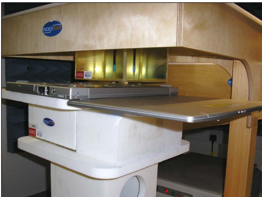
Figure 25: Positional Photograph of the Novatel U740 Wireless PCMCIA Card in Rear Facing Phantom Position using Host 1 – Averatec 6200 Series; 10mm Separation Distance
