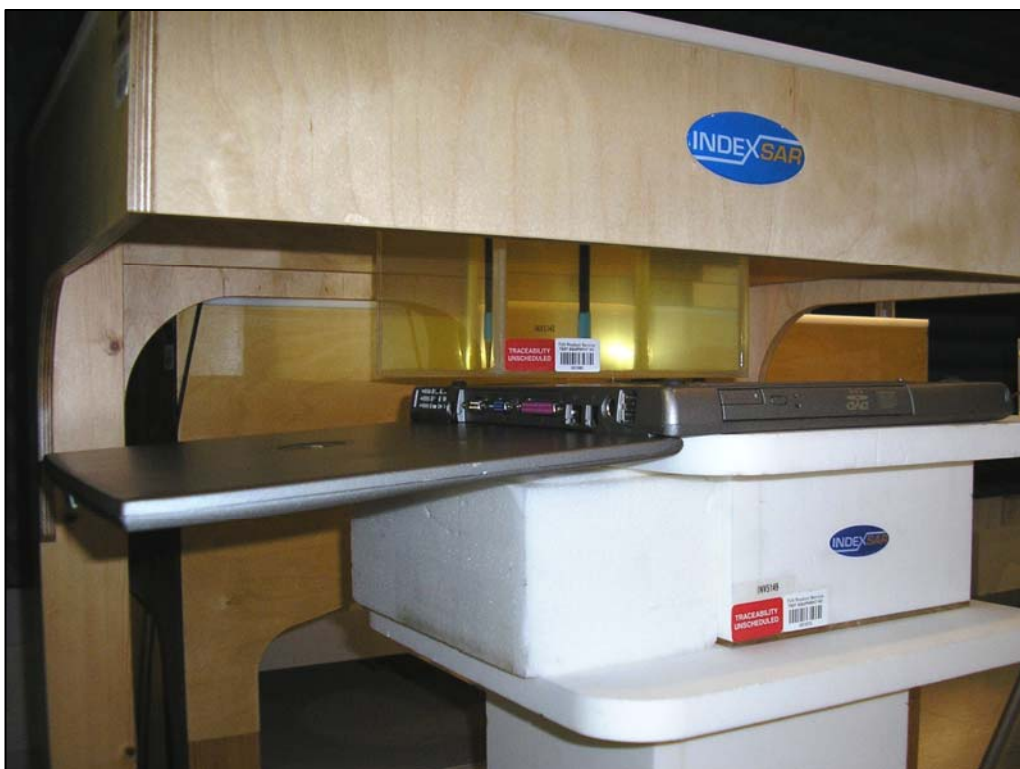
Figure 29: Positional Photograph of the Novatel U740 Wireless PCMCIA Card in Rear Facing Phantom Position using Host 3 – Dell Latitude D600; 14mm Separation Distance
