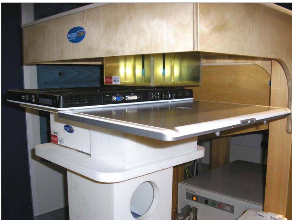
Figure 27: Positional Photograph of the Novatel U740 Wireless PCMCIA Card in Rear Facing Phantom Position using Host 2 – Dell Inspiron 9300; 18mm Separation Distance
