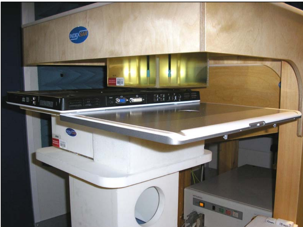
Figure 47: Positional Photograph of the Novatel U730 Wireless PCMCIA Card in Rear Facing Phantom Position using Host 2 – Dell Inspiron 9300; 18mm Separation Distance
