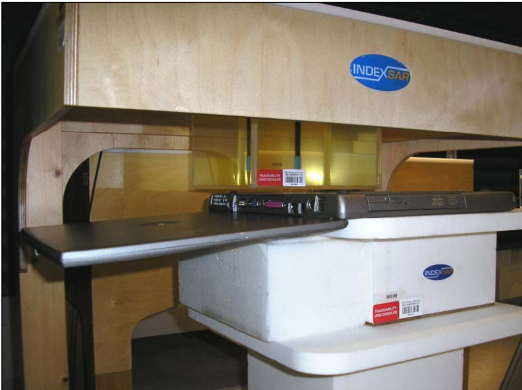
Figure 49: Positional Photograph of the Novatel U730 Wireless PCMCIA Card in Rear Facing Phantom Position using Host 3 – Dell Latitude D600; 14mm Separation Distance
