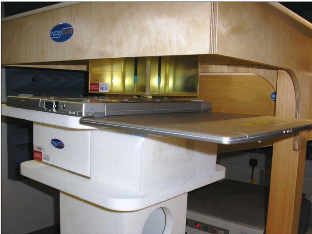
Figure 45: Positional Photograph of the Novatel U730 Wireless PCMCIA Card in Rear Facing Phantom Position using Host 1 – Averatec 6200 Series; 10mm Separation Distance
