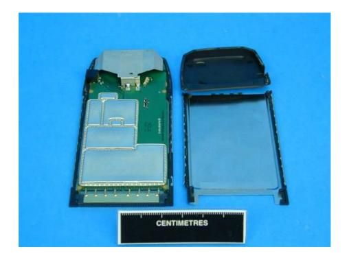
Merlin U703 Card – Top View with Shielding
