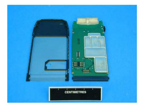
Merlin U703 Card - Bottom View with Shielding
