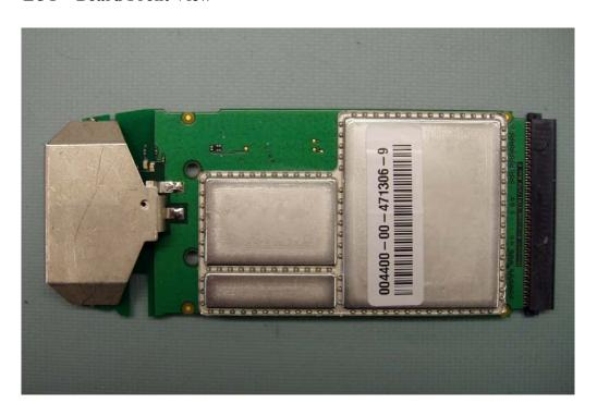
**EUT – Board Front Shield Off**
