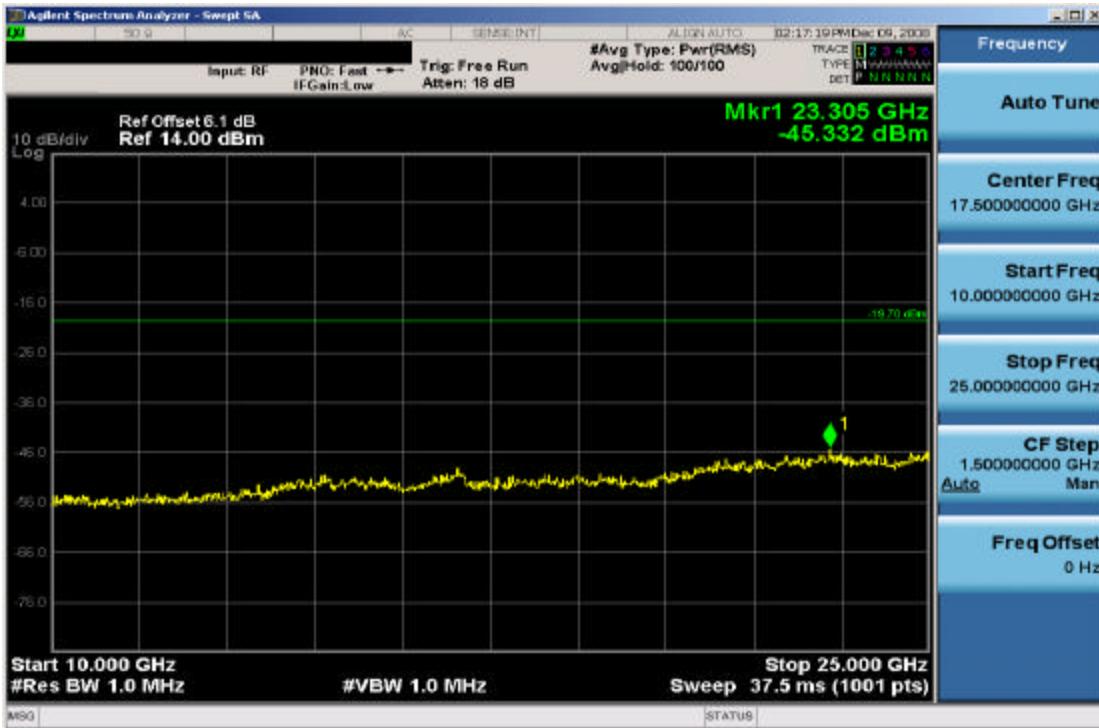
Plot 6-18. Conducted Spurious Plot (802.11b – Ch. 1)
