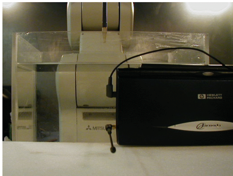
Figure S6. Position #6 Antenna perpendicular to the phantom with headset PCS 1900 MHz
