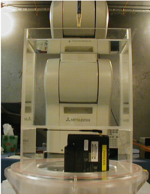
Figure S1. Position #1 - Antenna vertical and parallel to the phantom - PCS 1900 MHz
