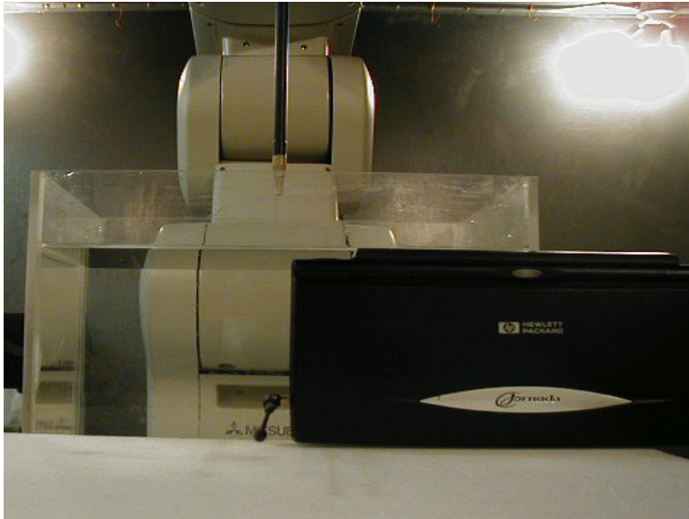
Figure S5. Position #5 Antenna perpendicular to the phantom without headset PCS 1900 MHz
