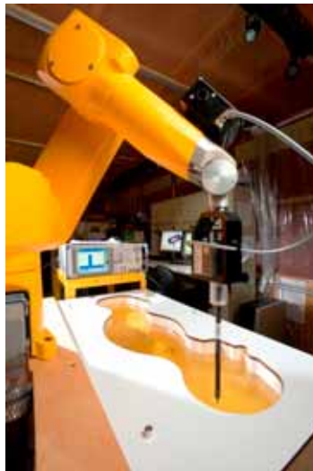
Figure 3-2 DASY4 SAR Measurement System
