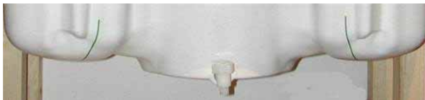
Figure 7-2 SAM Twin Phantom Shell
