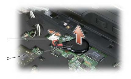
1 coin-cell battery connector 2 coin-cell battery
