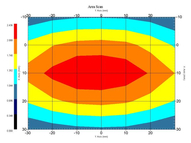
1 gram SAR value : 2.268 W/kg 10 gram SAR value : 1.486 W/kg Area Scan Peak SAR : 2.435 W/kg Zoom Scan Peak SAR : 3.413 W/kg
