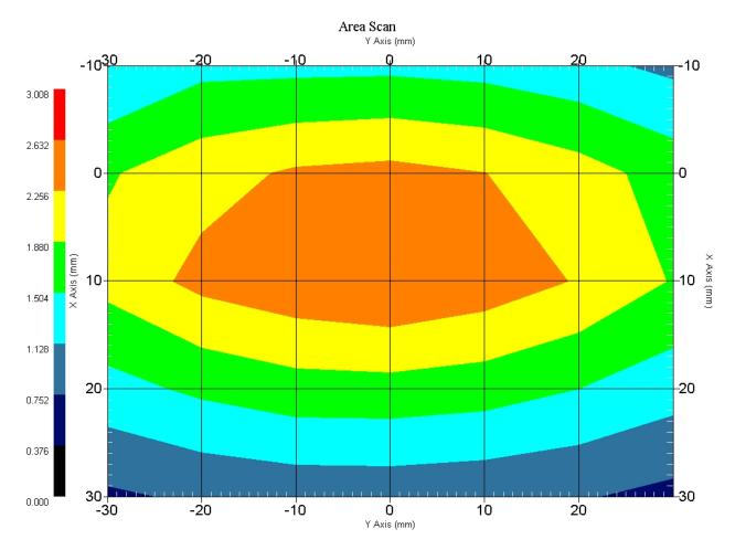
1 gram SAR value : 2.455 W/kg 10 gram SAR value : 1.590 W/kg Area Scan Peak SAR : 2.632 W/kg Zoom Scan Peak SAR : 3.693 W/kg
