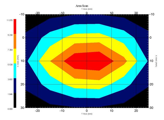
1 gram SAR value : 10.159 W/kg 10 gram SAR value : 5.106 W/kg Area Scan Peak SAR : 11.075 W/kg Zoom Scan Peak SAR : 17.815 W/kg
