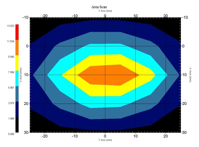
1 gram SAR value : 10.334 W/kg 10 gram SAR value : 5.366 W/kg Area Scan Peak SAR : 11.936 W/kg Zoom Scan Peak SAR : 18.616 W/kg
