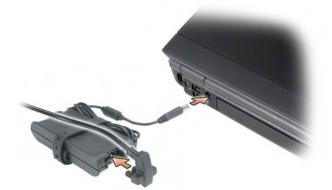
CAUTION: The AC adapter works with electrical outlets worldwide. However, power connectors and power strips vary among countries. Using an incompatible cable or improperly connecting the cable to the power strip or electrical outlet may cause fire or equipment damage.
