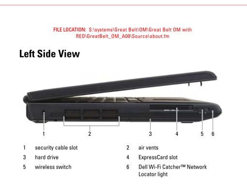
**SECURITY CABLE SLOT** — Lets you attach a commercially available antitheft device to the computer (see "Security Cable Lock" on page 95).
