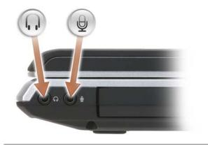
Attach headphones to the \(\int\_{\text{\text{\connector.}}}\) connector.
