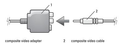
**4** Plug the other end of the composite video cable into the composite video-input connector on the TV.
