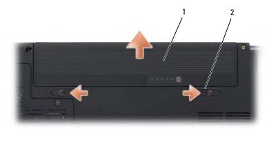
1 battery 2 battery release latches (2)
