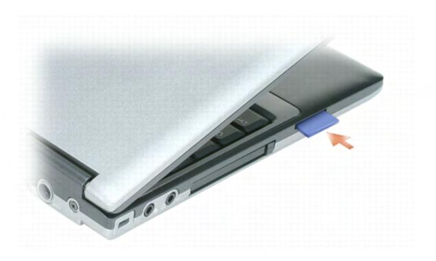
To remove a secure digital card, press in on the card and it will spring outward. Remove the card from the computer.
