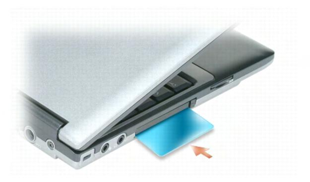
To remove a smart card, slide the card out of the computer.
