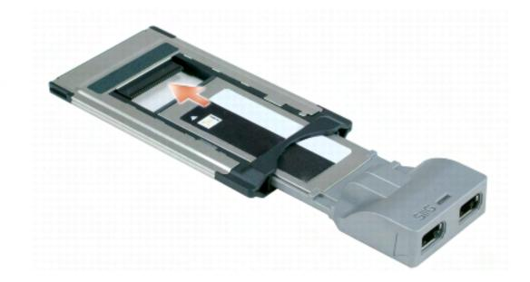
2. Install the ExpressCard with adapter the same way as a PC Card. See Installing a PC Card.
