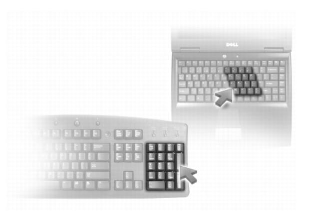
The numeric keypad functions like the numeric keypad on an external keyboard. Each key on the keypad has multiple functions. The keypad numbers and symbols are marked in blue on the right of the keypad keys. To type a number or symbol, hold down <Fn> and press the desired key.
